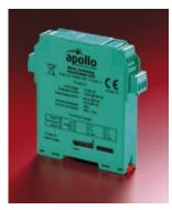
accept wires up to 2.5 mm<sup>2</sup>. The unit has dimensions of 110 x 107 x 20 mm and weighs 95g. It has been designed to comply with EN54-18. The mains switching input/output unit is loop-powered and can only operate with control equipment using the company's XP95 or Discovery protocols. Application examples include air sampling units, mains power shut-down on machinery, automatic door retainers, smoke dampers and gas valves.
