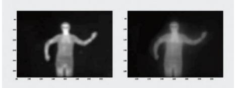
Comparison of IR images produced through a Trifocus lens (left) and conventional mirror (right)
