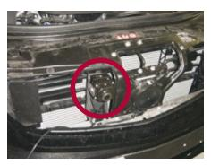
The FLIR Systems PathFindIR installed behind the vehicle grid of an armored Mercedes.
