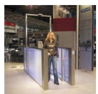
pose, any standard document reader and biometrical device can be applied. As an additional feature, the company's ABC system is equipped with an infrared sensor to detect that just one person at a time is inside the interlock – an essential requirement for reliable border control. The units for Automated Border Control are currently operating in a number of pilot projects in European airports.
