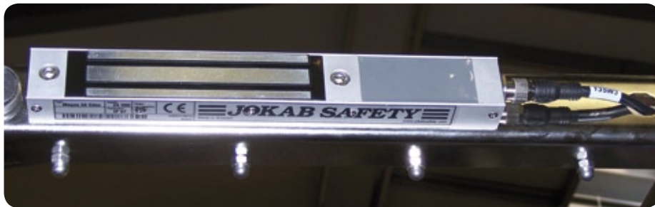
Fig. 2. The magnetic lock Magne 2 with integrated safety sensor Eden can hold a door closed electrically with a force of up to 1500 Newtons.
