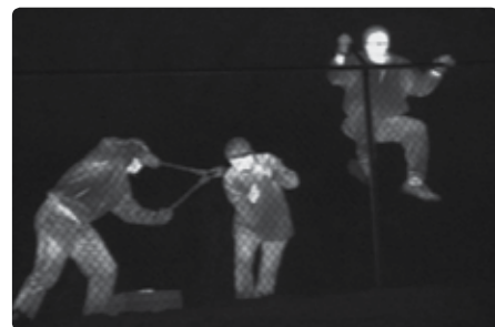
Intruders are easily spotted by thermal imaging cameras. No need to install expensive lighting
