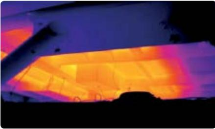
Fig. 2: Infrared picture of a steel structure affected by heat exposure from above. The yellow areas are hottest and the blue areas are coldest.
