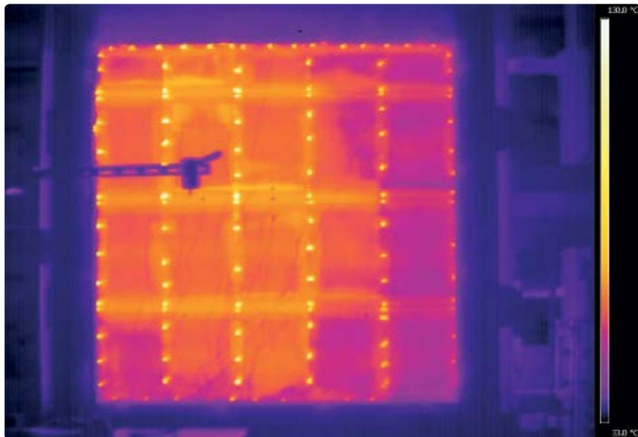
Fig. 1: The infrared camera was used during a test of a non load-bearing wall with steel beams and two layers of normal plaster on each side. The infrared picture clearly shows distinct hot spots where the plaster boards are fixed to the beams (the light yellow dots).
