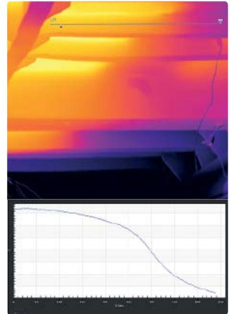
Fig. 3: An infrared picture of steel beams, where yellow areas are hot and blue areas are cold. On one of the beams there is a distinct line. A detailed temperature overview along this line is shown in the bottom picture where the y axis shows the temperature and the x axis shows the line on the steel beam. The graph is taken from an analysis in the camera software.
