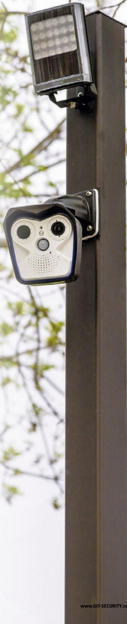
located in the exact area of concern, is configured to produce a solid-on White-Light output to allow the 5MP Mobotix optical camera in that area to generate a detailed night time colour image of the intruder for identification; displayed both on-site and streamed live off-site to the central video monitoring station.
