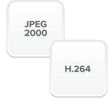
As a temporal compression standard, H.264 inherently attempts to store only incremental changes between frames and whole frames at periodic intervals. The result is a stream of video that is compressed over multiple frames rather than a series of individual frames, as in JPEG2000.
