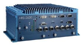
A complete system for passenger information and video surveillance built around this rugged mobile PC and known as the ITA 5000 can be obtained from Advantech
