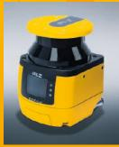
safety laser scanner can now also be used for dynamic navigation of automated guided vehicles or generally for mobile applications in robotics, using SLAM for example (Simultaneous Localisation and Mapping). The required ROS packages can be installed directly from the open source framework, which makes integration easier. Pilz's own development of the software features by Pilz itself also ensures that they are quickly available to the user.
