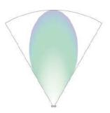
1D-Radar (CW): Measures only one parameter (velocity) and can therefore not localize objects
