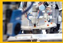
has designed a fully automated test system. For 225 variants the robot is measuring the threads, the forcedistance ratio and the torque, a visual inspection is done simultaneously by cameras. By means of the serial number, which the robot prints on automatically and the inspection record the result's traceability is always guaranteed. In cooperation with all departments involved the requirements for the testing system were documented in a specification sheet.
