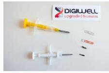
The small x-series tags are placed directly beneath the skin using a cannula. The flat flex implants, by contrast, should be inserted by an experienced body modder or doctor
